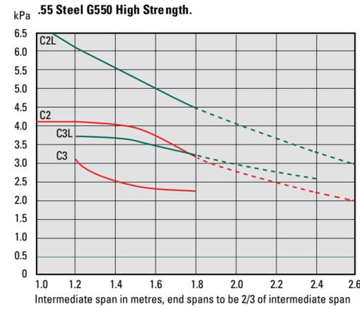
C2L, C3L, C2 and C3 represent alternative primary fixing methods. The dotted lines indicate purlin spans only suitable for non accessible roof areas and wall cladding. Testing confirms that .70mm Aluminium has similar results to .40mm Steel and that .90mm Aluminium has similar results to .55mm Steel and is adjusted for practical application. Aluminium requires load spreading washers and EPDM washers at all times. For compliance with NZ Metal Roof and Wall Cladding Code of Practice.
